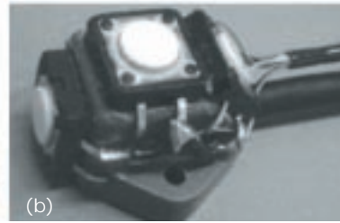
1 (a) Using SFA's two-handed stereo interface. (b) A 3D tracker with buttons attached.
